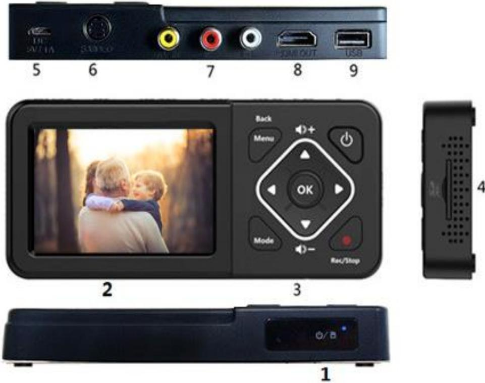
1. **LED indicators:** A blue light means the device is on. A blue blinking light means it is running low on memory.
